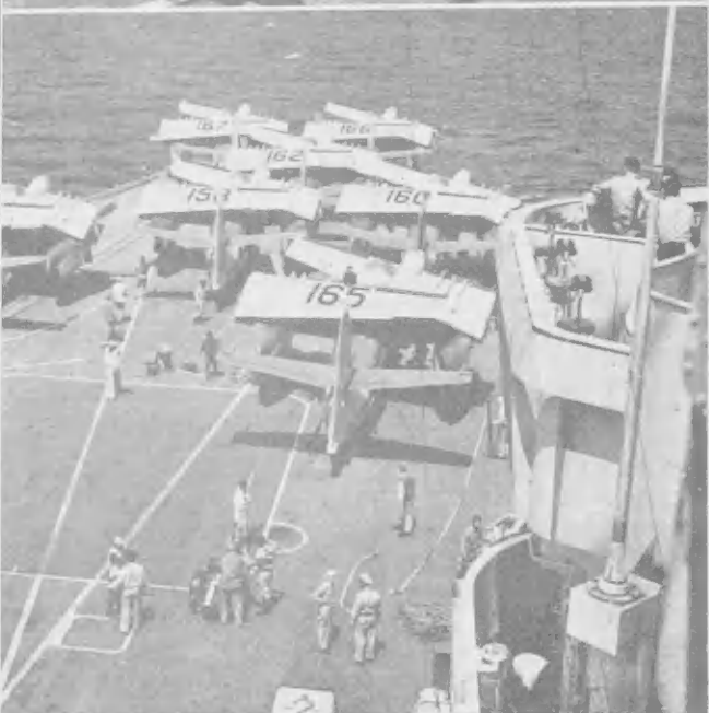
ACTIVITIES are graphically depicted in this cluster of pictures. The ship's twelve Trackers touches down, catches its tail arresting cable strung across the flight deck, decelerates and folds its wings. The canted deck allows the plane that is able to continue on, below, rather than risk the possibility of collision with the planes parked at the end of the flight deck, above.
